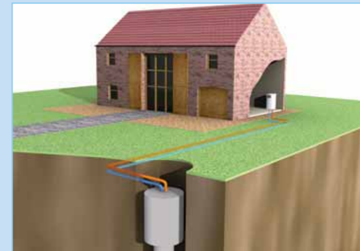
Bore hole collector
